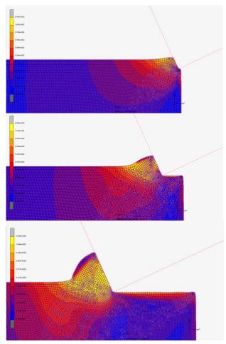
Fig. 5. Chip formation for rake angle  $-10^{\circ}$  for cutting speed 180 m/min and undeformed chip thickness 0.01 mm.
