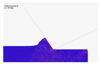
Fig. 6. Chip formation for rake angle  $-35^{\circ}$  for cutting speed 180 m/min and undeformed chip thickness 0.01 mm.
