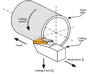
Fig. 1. Experimental setup for orthogonal cutting
