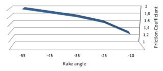
Fig. 7. Effect of tool rake angle on friction coefficient.
