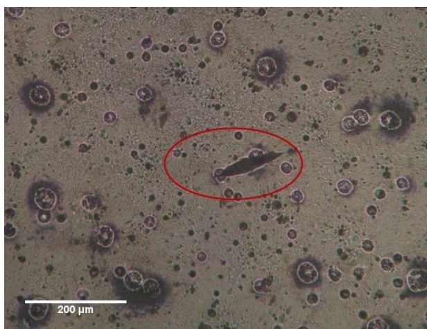
Fig. 3a. Shows impression remaining in the studied sample with coating thickness 120.27 μm and Knoop micro hardness number is 13.85 KHN.
