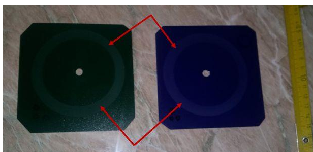
Fig. 4. Remain effect of the abrasive wear on the polyurethane film coating on coated samples.
