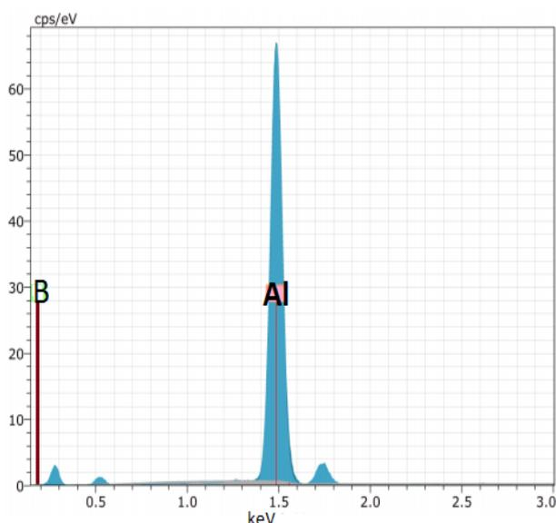
**Figure 4.** EDS analysis of LM25/AlB<sub>2</sub>.
