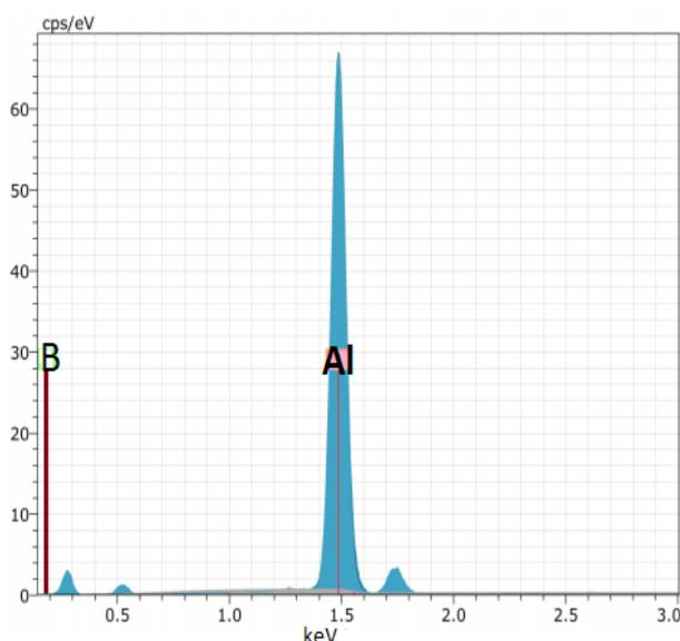
**Figure 4.** EDS analysis of LM25/AlB<sub>2</sub>.
