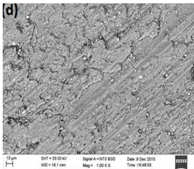
**Fig. 3.** Worn out surface analysis at various conditions a) L = 10N, V = 1m/s, S.D = 400m b) L = 10N, V = 2m/s, S.D = 800m c) L = 10N, V = 4m/s, S.D = 1600m d) L = 30N, V = 1m/s, S.D = 1200m.
