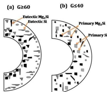
**Fig. 18.** Particles segregation mechanisms under effect of G-Factor.
