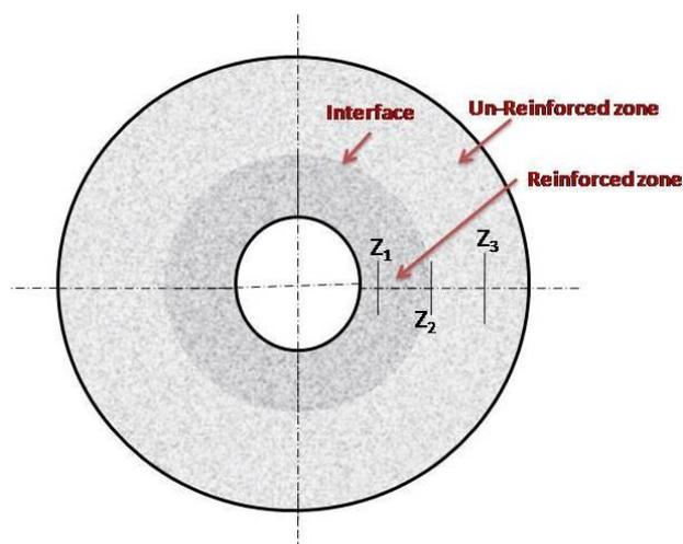
**Fig. 3.** Schematic representation of the different zones characterized from the geometrical centre of the sample: ( $Z_1=40$  mm, ( $Z_2= 46$  mm) and ( $Z_3=50.5$  mm).
