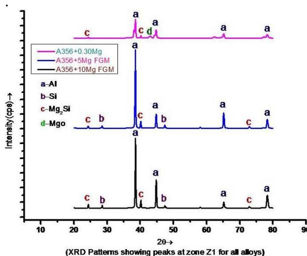
**Fig. 5.** XRD pattern showing the clear peaks of phase particles for each alloys (a) A356 Alloy, (b) A356+5Mg at 1200 rpm and (c) A356+10Mg at 1600 rpm.
