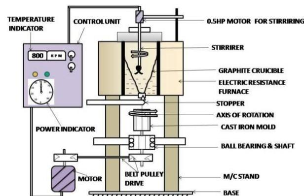
**Fig. 1.** Schematic illustration of the centrifugal casting process set-up.
