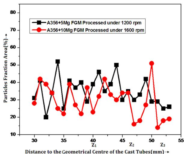
**Fig. 6.** Distribution of the  $Mg_2Si$  particles fraction area as a function of the distance to the geometrical centre for both FGM's cast at 1200 and 1600 rpm.
