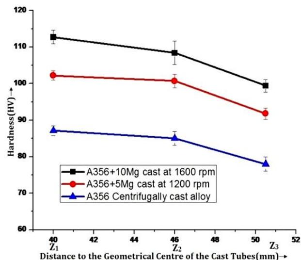
**Fig. 11.** Hardness evolution as function of the distance to the geometrical centre of the FGM tube for both FGM's cast at 1200 and 1600 rpm and A356 alloy cast at 1200 rpm.
