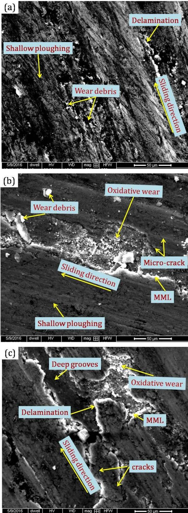
**Fig. 15.** SEM micrographs of worn surfaces with load variations (a) A356 alloy, (b) A356+5Mg FGM and (c) A356+10Mg FGM at  $Z_1$ .
