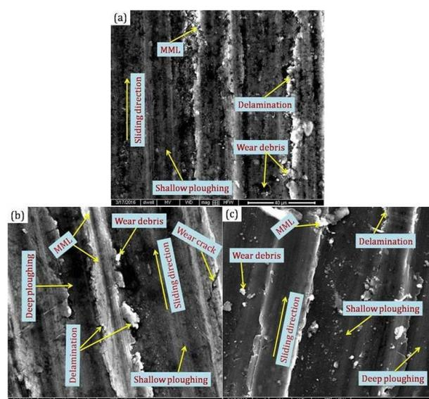
**Fig. 13.** SEM micrographs of worn surfaces at constant load (40 N) for (a) A356 alloy, (b) A356+5Mg FGM and (c) A356+10Mg FGM at Z<sub>1</sub>.
