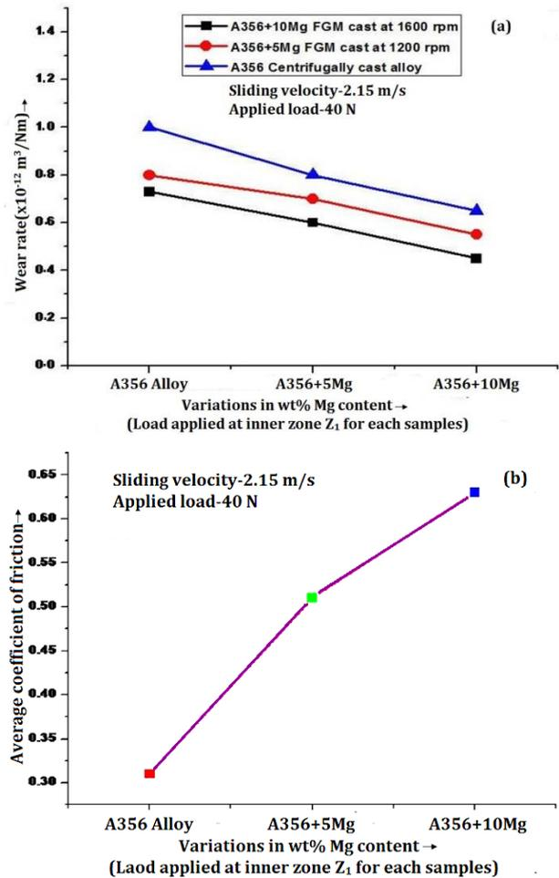
**Fig. 16.** Effect of constant load on (a) wear rate (b) average COF with variations of Mg contents.
