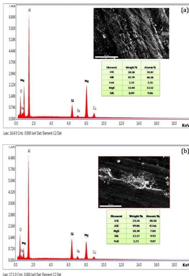
**Fig. 17.** SEM morphology of wear surface at load 40N and EDS spectrum for both FGMs (a)A356+5Mg processed under 1200rpm (b)A356+10Mg processed under 1600 rpm at inner zone Z<sub>1</sub> of geometrical tube.
