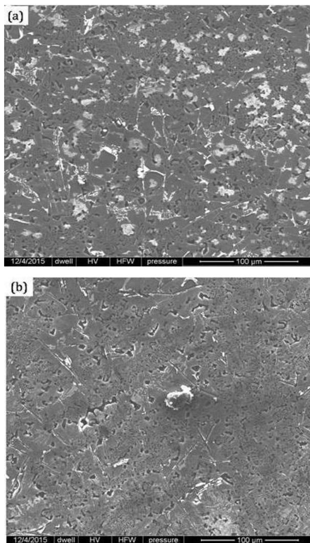
**Fig. 7.** SEM micrographs of the centrifugally cast FGMs (a) A356+5Mg processes under 1200 rpm and (b) A356+10Mg FGMs processes under 1600 rpm observed at: inner zone  $Z_1$  of the rings.
