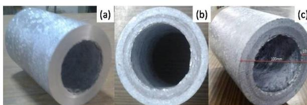
**Fig. 2.** Centrifugally cast Alloy/FGMs obtained as (a) A356 Alloy, (b) A356+5.0Mg processed at 1200 rpm and (c) A356+10.0Mg processed at 1600 rpm.
