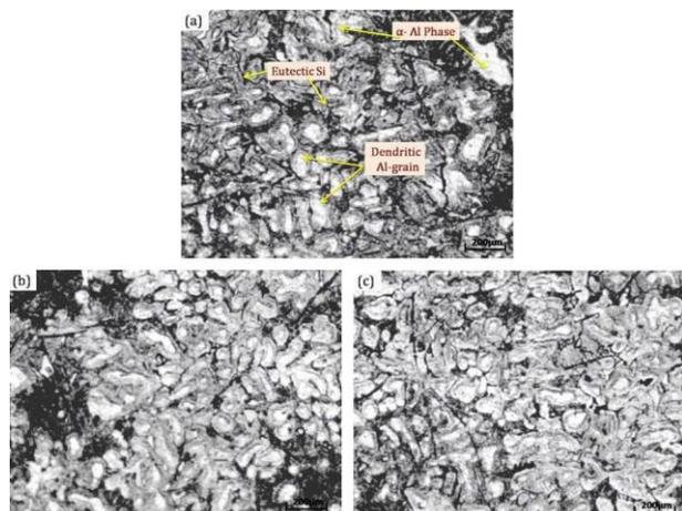
**Fig. 8.** Optical micrographs of the A356 alloy processed under 1200rpm at (a) Inner zone  $Z_1$ , (b) Middle Zone  $Z_2$  and (c) outer zone  $Z_3$ .
