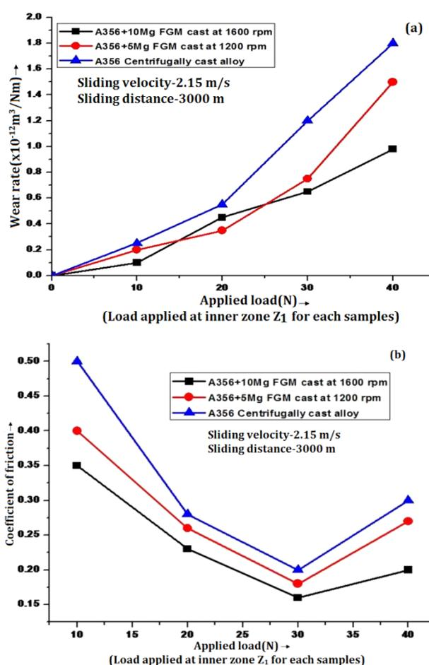
**Fig. 14.** (a) Variation of wear rate with applied load and (b) Variation of COF with applied load for both FGMs processed under 1200 rpm and 1600 rpm and A356 alloy processed under 1200 rpm.
