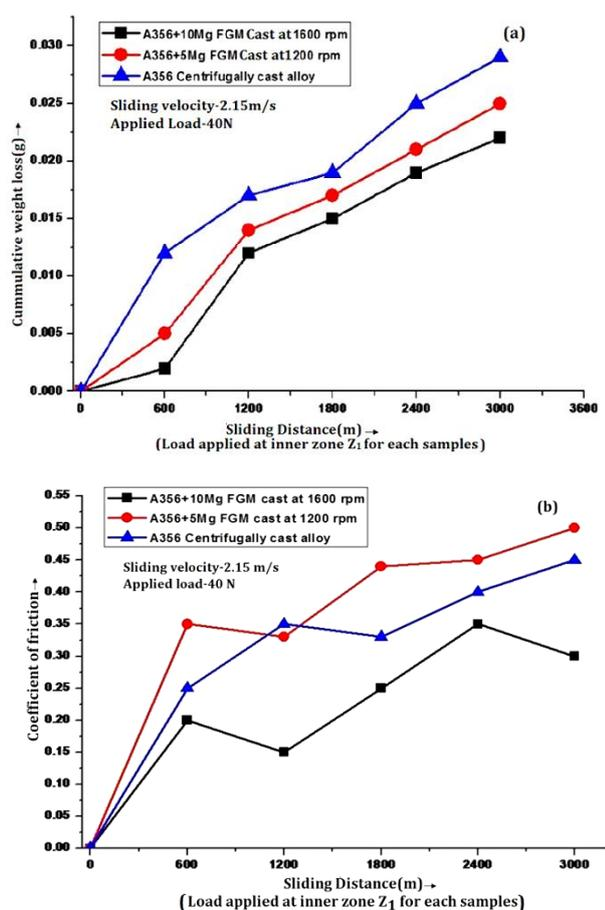
**Fig. 12.** Variation of (a) cumulative wt. loss and (b) COF with sliding distance(m) at zone Z<sub>1</sub>(inner core) to the geometrical centre of the FGM tube for both FGM's cast at 1200 and 1600 rpm and A356 alloy cast at 1200 rpm.
