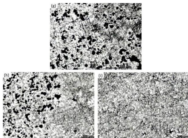
**Fig. 10.** Optical micrographs of the A356+10Mg FGM's processed under 1600 rpm at (g) Inner zone  $Z_1$ , (h) Middle Zone  $Z_2$  and (i) outer zone  $Z_3$  from geometrical centre of tubes.
