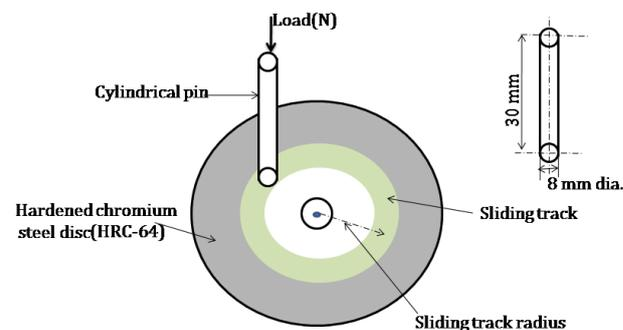
**Fig. 4.** Schematic illustration of pin-on-disc type tribometer.
