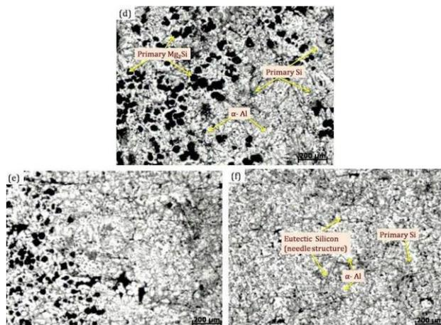
**Fig. 9.** Optical micrographs of the A356+5Mg FGM's processed under 1200rpm at (d) Inner zone  $Z_1$ , (e) Middle Zone  $Z_2$  and (f) outer zone  $Z_3$ .
