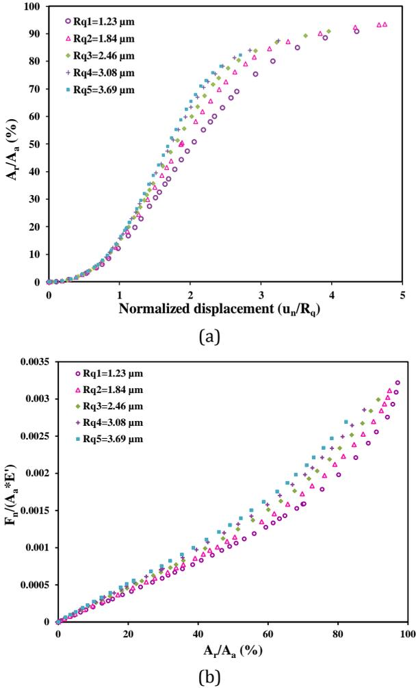
**Fig. 9.** (a) Variation of the area ratio with normalized displacement for the elastic-plastic model, (b) Normalized load versus contact area ratio.
