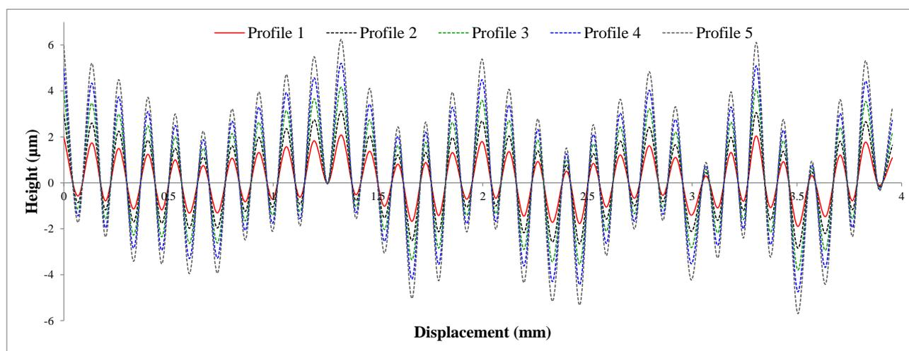
Fig. 2. Profiles of the simulated rough surfaces.
