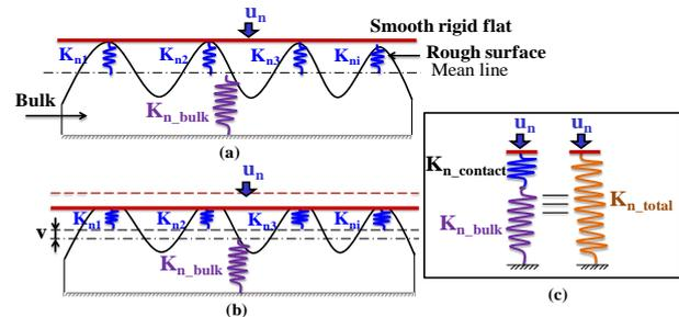
**Fig. 6.** Spring model representation: (a) before loading (b) after loading (c) equivalent rheological model.
