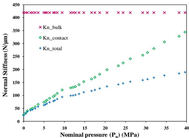
**Fig. 7.** Evolution of contact stiffness, bulk stiffness and total stiffness as a function of nominal pressure for profile 1.
