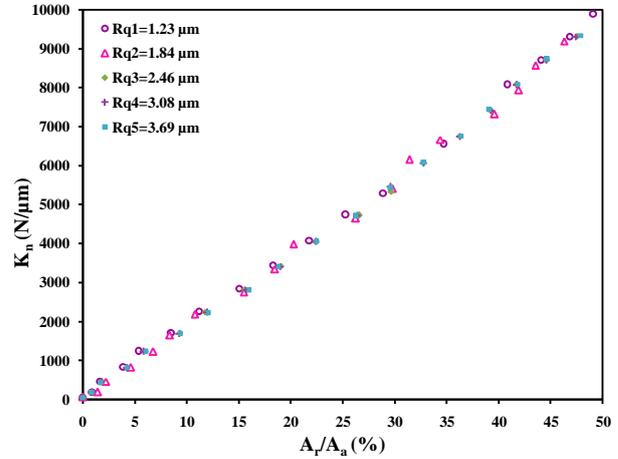
**Fig. 8.** Contact stiffness of elastic contact versus the area ratio.
