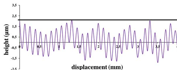
Fig. 1. Investigated contact: Surface profile-flat plan.
