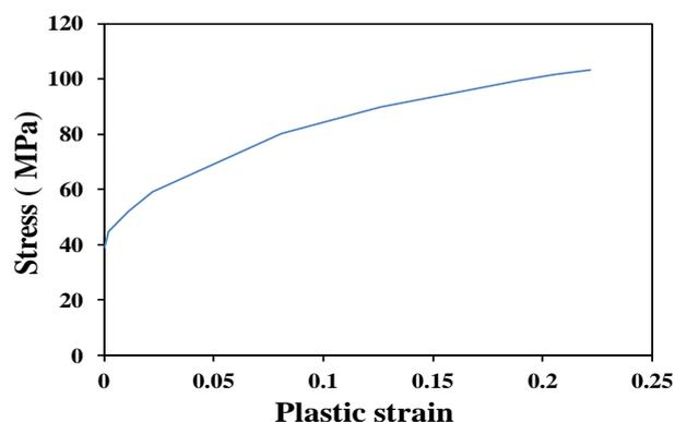
Fig. 4. The power-law hardening curve.
