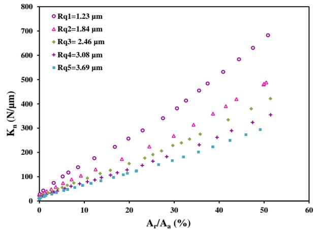
**Fig. 10.** Contact stiffness against area ratio for the elastic-plastic model.
