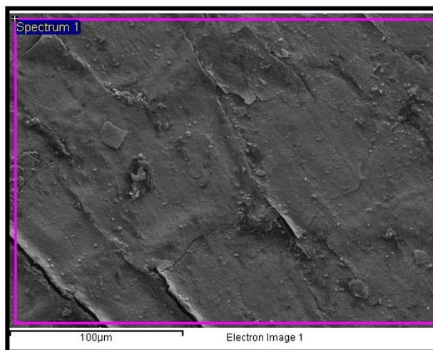
**Fig. 6.** SEM image showing the topography of electroless Ni-P film morphology (cracks and roughness) on PP surface (x1000).
