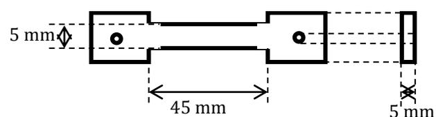
**Fig. 1.** Polypropylene specimens used for the experiment.
