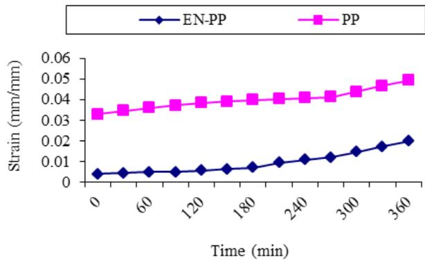
**Fig. 13.** Creep test of EN-PP and PP under 5 kg load.
