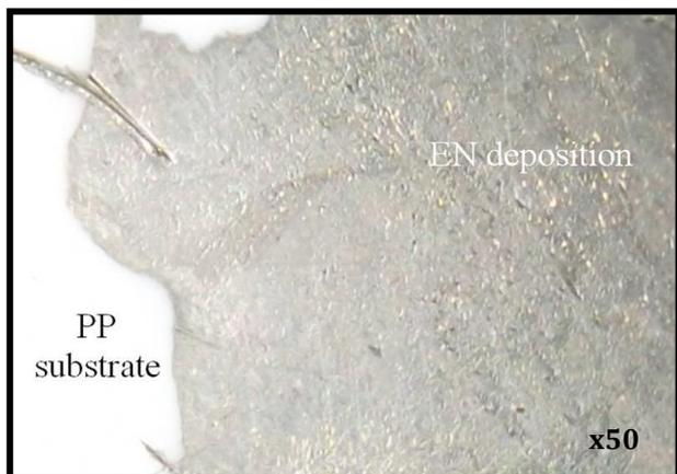
**Fig. 4.** Photomicrograph showing adhesion at interface of bright metallic electroless Ni deposition on PdCl<sub>2</sub> activated PP plastic (x50).
