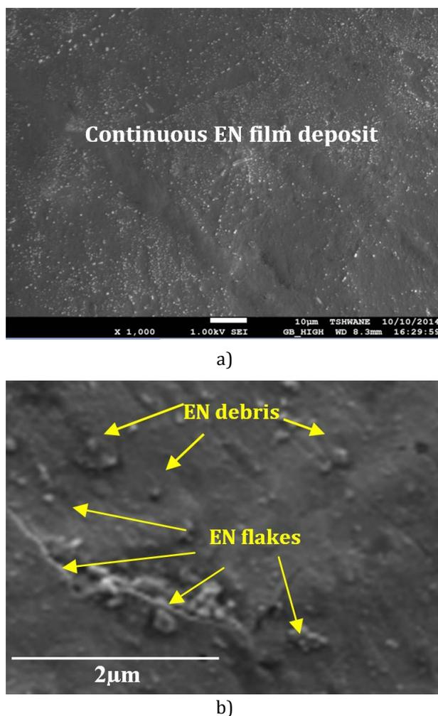
**Fig. 3.** SEM image showing (a) the continuity electroless EN film and (b) EN flakes on PdCl<sub>2</sub> activated PP substrate (x1000)
