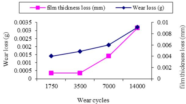
**Fig. 10.** Wear loss and film thickness loss due to abrasive wear test using P600 grit.
