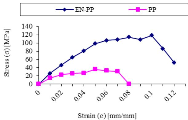
**Fig. 12.** Strength test of EN-PP and PP.
