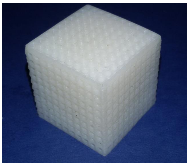
Fig. 2. Porous polymer scaffold aimed for tissue engineering - seeding of 3D cell culture, fabricated by additive manufacturing technology, Fused deposition modeling (FDM) (Faculty of Engineering Kragujevac, Serbia).
