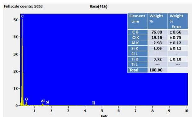
Fig. 9. Energy dispersive X-ray analysis (EDXA) of MCD Coatings.
