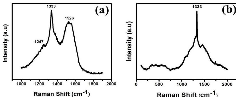
Fig. 2. Raman spectra of CVD-diamond coatings, (a) NCD and (b) MCD.
