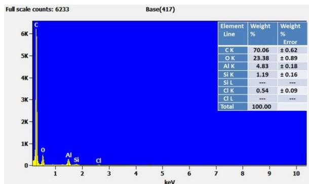
Fig. 10. Energy dispersive X-ray analysis (EDXA) of NCD Coatings.
