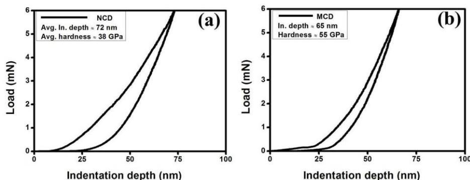
Fig. 3. (a) Load-displacement curve for NCD coating, (b) Load-displacement curve for MCD coating.
