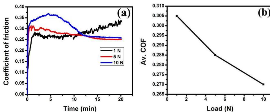
Fig. 5. Tribological characteristics of MCD coatings sliding against alumina ball. (a) Coefficient of friction vs duration of rubbing at 1 N, 5 N and 10 N, (b) Average coefficient of friction vs. normal load.
