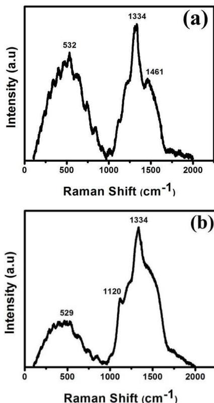
Fig. 8. Raman spectra of wear track of CVD-diamond coatings, (a) NCD and (b) MCD.
