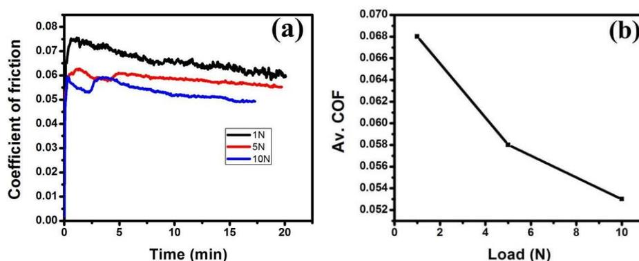
Fig. 6. Tribological characteristics of NCD coatings sliding against alumina ball, (a) Coefficient of friction vs duration of rubbing at 1 N, 5 N and 10 N, (b) Average coefficient of friction vs. normal load.
