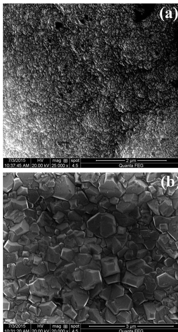
**Fig. 1.** CVD-diamond coatings, (a) Surface morphology of NCD coatings, (b) Surface morphology of MCD coatings.
