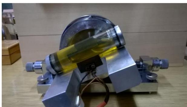
Fig. 3. Rotating the platform and begin sliding the pin.
