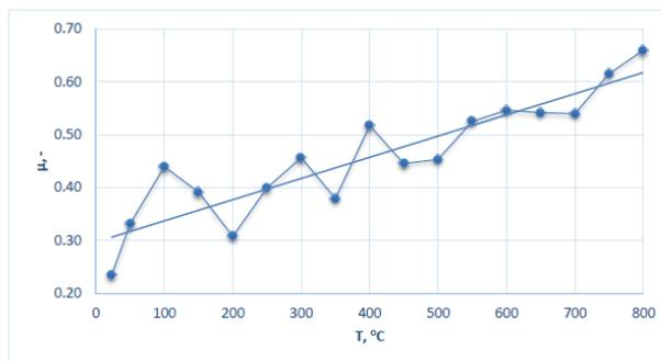
Fig. 4. Dependence of the static coefficient of friction  $\mu_s$  from the previous preheating temperature T.
