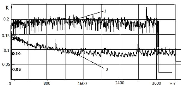
Fig. 5. Friction coefficient oscillograms: 1 – oil I-20A; 2 – oil I-20A with AWAF composition (the friction pair steel10 – steel10).
