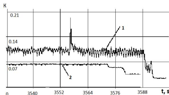
**Fig. 2.** Friction coefficient oscillograms: 1 – lubricant Soliton, 2 – lubricant Soliton with AWAf.
