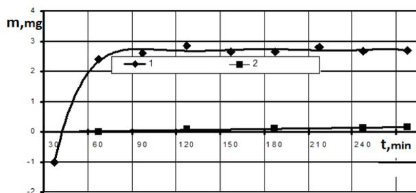
Fig. 4. Weight change of the roller (1) and plate (2) depending on the processing time (the friction pair steel10 – steel10).
