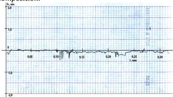
Fig. 6. The profilograms of friction surfaces of the parts samples.
