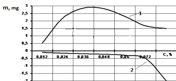
Fig. 3. Weight change of the roller (1) and plate (2) depending on the concentration of the AWAF composition (the friction pair steel10 – steel10).
