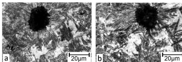
**Fig. 6.** Upper bainite in austempered ductile irons: a-sample 5; b-sample 6.
