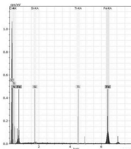
**Fig. 3.** EDX analysis of the graphite phase in spheroidal graphite cast irons with nanoadditives of TiCN+TiN (sample 2).
