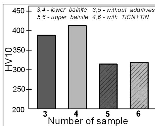
Fig. 7. Hardness HV10 of austempered ductile irons with a lower bainitic structure (samples 3 and 4) and upper bainitic structure (samples 5 and 6).
