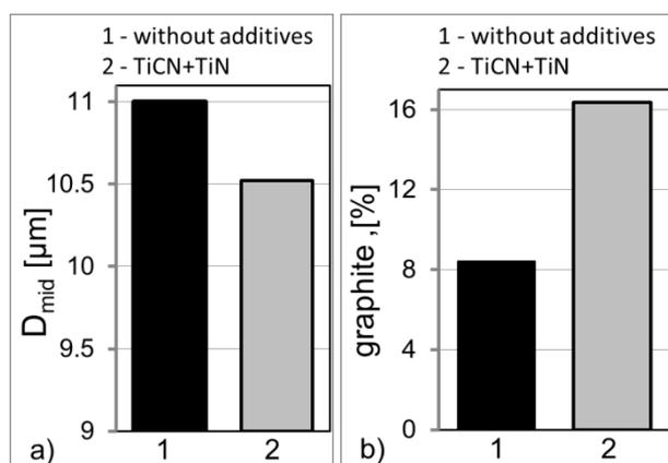
**Fig. 1.** Average diameter of the graphite spheres  $D_{mid}$  (a) and graphite quantity (b) in spheroidal graphite cast irons: samples number - 1 and 2.
