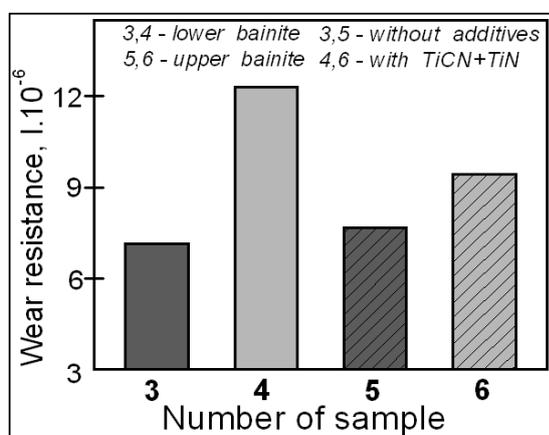
**Fig. 9.** Wear resistance  $I$  of austempered ductile irons with a lower bainitic structure (samples 3 and 4) and upper bainitic structure (samples 5 and 6).
