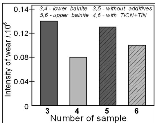
**Fig. 8.** Intensity of wear  $i$  of austempered ductile irons with a lower bainitic structure (samples 3 and 4) and upper bainitic structure (samples 5 and 6).
