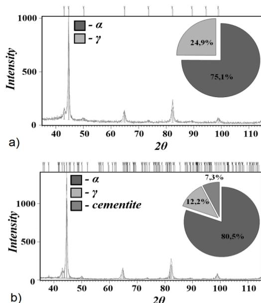
Fig. 11. X-ray diffraction pattern of austempered ductile iron sample 4 before (a) and after (b) wear test.
