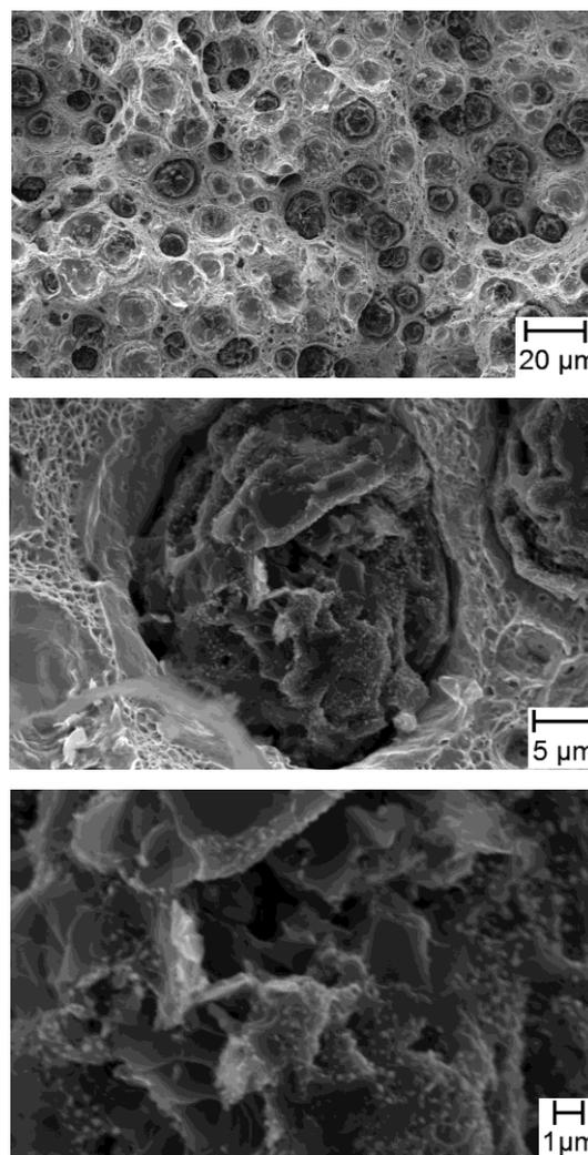
**Fig. 2.** SEM analysis of the fracture of the impact destructive sample from spheroidal graphite cast irons with nanoadditives of TiCN+TiN (sample 2).
