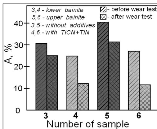
**Fig. 10.** Quantity of the retained austenite  $A_i$  of austempered ductile irons with a lower bainitic structure (samples 3 and 4) and upper bainitic structure (samples 5 and 6) before and after tribological testing.
