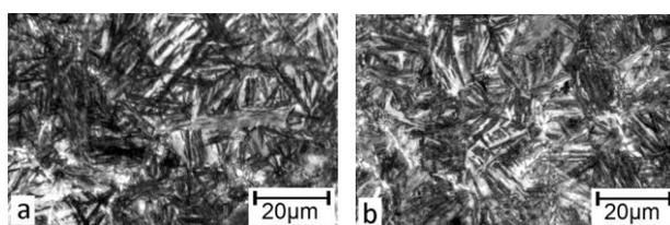
**Fig. 5.** Lower bainite in austempered ductile irons: a-sample 3; b-sample 4.
