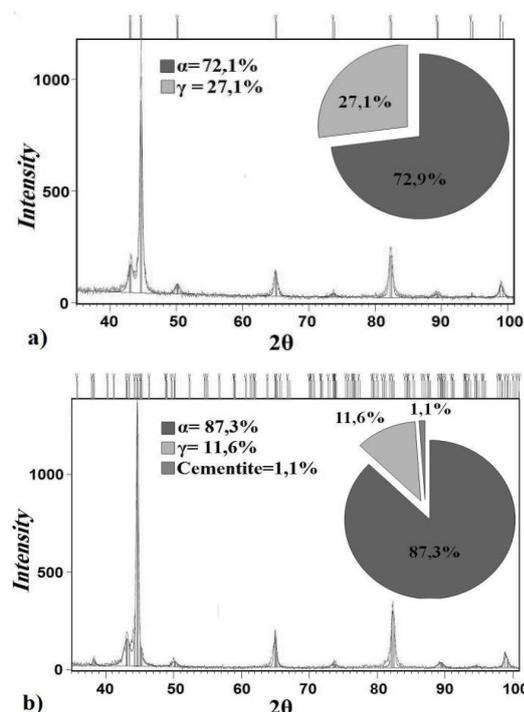
Fig. 12. X-ray diffraction pattern of austempered ductile iron sample 6 before (a) and after (b) wear test.
