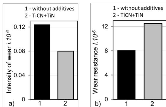
**Fig. 4.** Intensity of wear  $i$  (a) and wear resistance  $I$  (b) of spheroidal graphite cast irons: samples number – 1 and 2.
