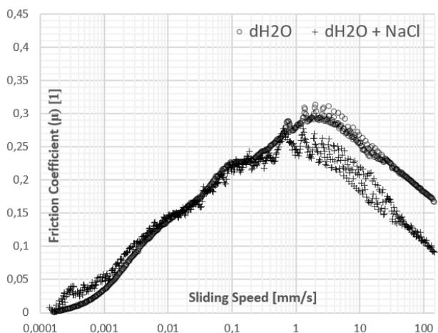
**Fig. 11.** Compiled result for different lubricants interacting with Condyle samples with a 10 N normal force.
