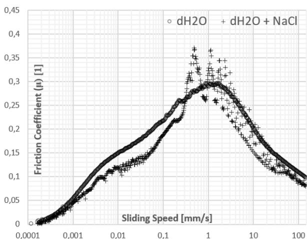
**Fig. 10.** Compiled result for different lubricants interacting with Condyle samples with a 5 N normal force.
