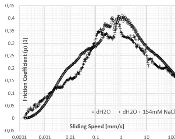
**Fig. 8.** Compiled result for different lubricants interacting with Plateau samples with a 5 N normal force.
