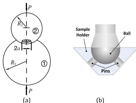
**Fig 7.** Contact area between two spheres. (a) Standard case (adopted from [21]) and (b) Ball-on-plates case (adopted from [15]).
