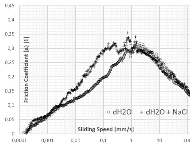
**Fig. 9.** Compiled result for different lubricants interacting with Plateau samples with a 10 N normal force.
